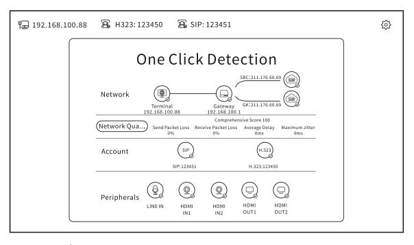
Step 2 Press the "<sup>()</sup>" key on remote control to save and return to the upper-level interface.
