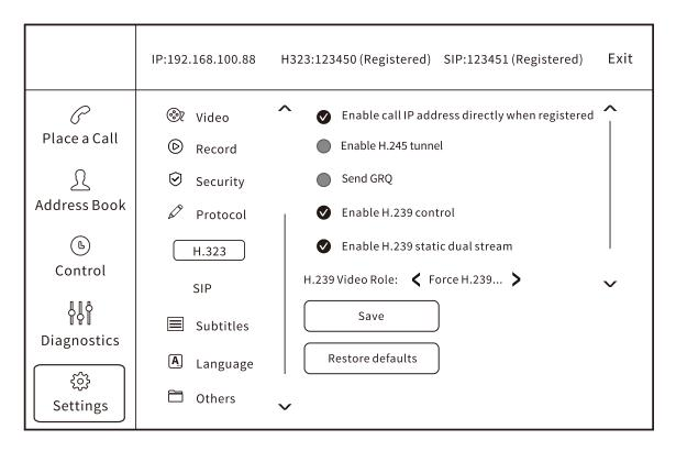
Step 2 Configure the "H.323 Protocol" parameters, which are shown in the table below.
