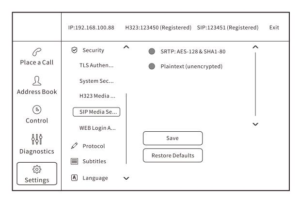
Step 2 Configure the "SIP Media Security" parameters, which are shown in the table below.
